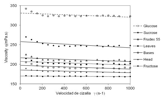
Figure 3. Viscosity vs. shear rate of the different syrups at 70°Brix and 25°C.
