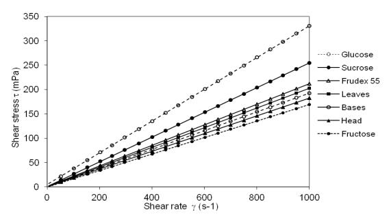
Figure 2. Shear stress vs. shear rate of the different syrups at 70°Brix and 25°C.
