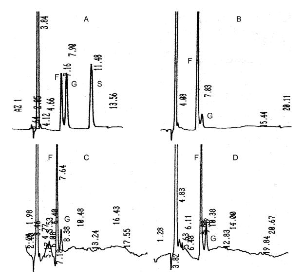
**Figure 1.** HPLC spectra of: A, Standards of fructose (F), glucose (G) and sucrose (S); B, Agave head syrup; C, Agave bases syrup; D, Agave leaves syrup.
