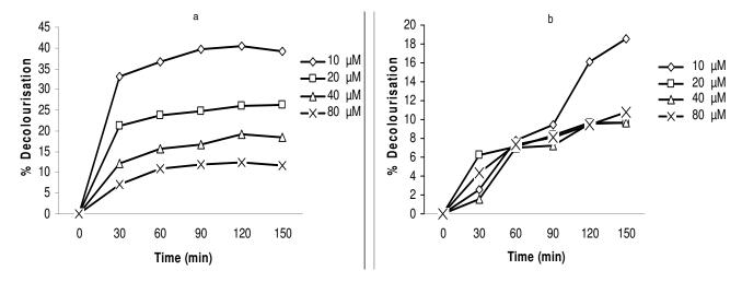
**Figure 6.** Indigo carmine decolourisation percentages at various initial dye concentration in 100 mM phosphate—citrate buffer, pH 5.0 by unboundLac, 0.01 U (a) and pH 3.0 by pool2Lac, 0.01 U.
