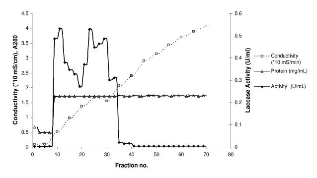
Figure 2. DEAE-cellulose elution profiles with two peaks of laccase activity observed.
