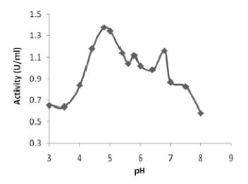
**Figure 2.** Optimum endoglucanase activity was observed in the acidic range at pH 4.8 and second peak was observed at 6.8 which is pH of insect gut. After pH 6.0 enzyme activity was declined abruptly.
