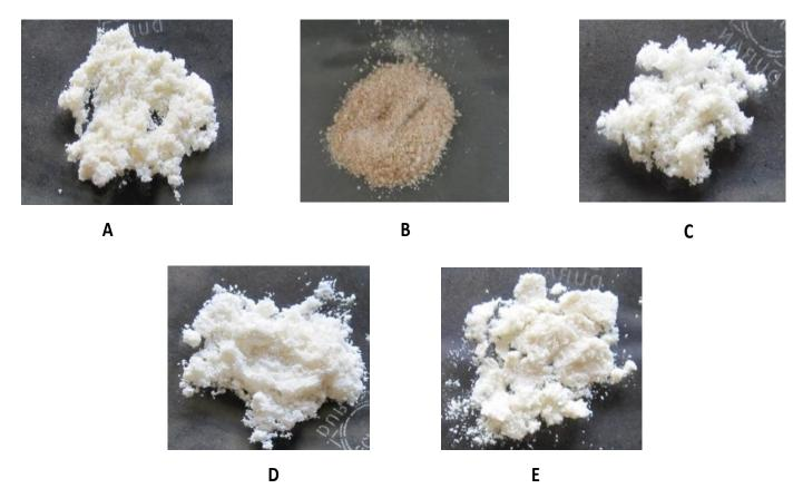
Figure 1. (A) Powder chitin. (B) Colloidal chitin. (C) Superfine chitin. (D) Amorphous chitin. (E) Bead chitin.
