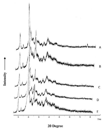
$\begin{tabular}{ll} \textbf{Figure 3.} & \textbf{Difractograme of powder chitin (A), colloidal chitin (B),} \\ & \textbf{amorphous chitin (C), bead chitin (D) and superfine chitin (E).} \\ \end{tabular}$
