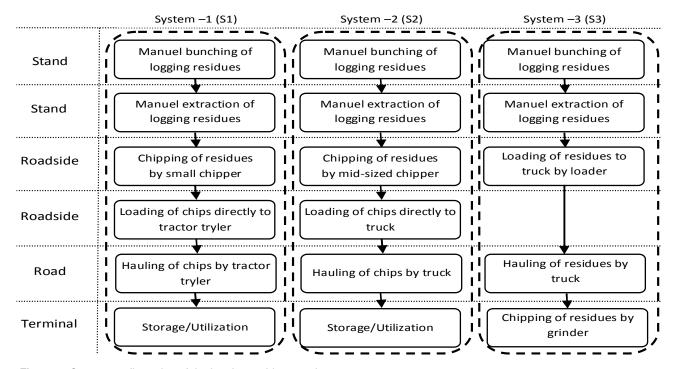
Figure 1. System configuration of the logging residue supply system.
