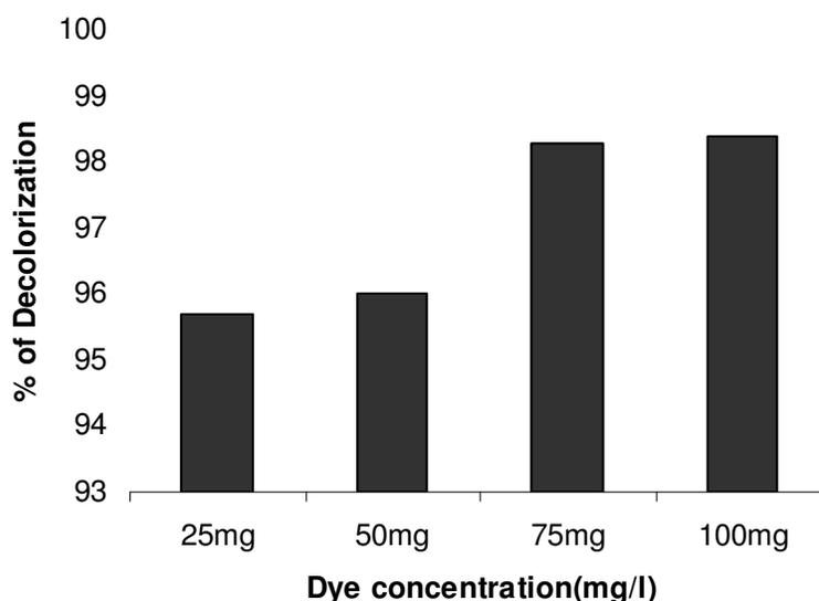
Figure 3. Effect of Reactive Blue dye concentration on decolorization by *Aspergillus* sp.
