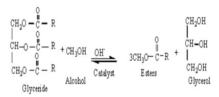
Figure 1. Transesterification reaction.
