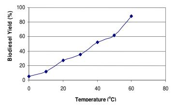
Figure 2. Effect of temperature on conversion of peanut oil to biodiesel at 1:6 molar ratio.
