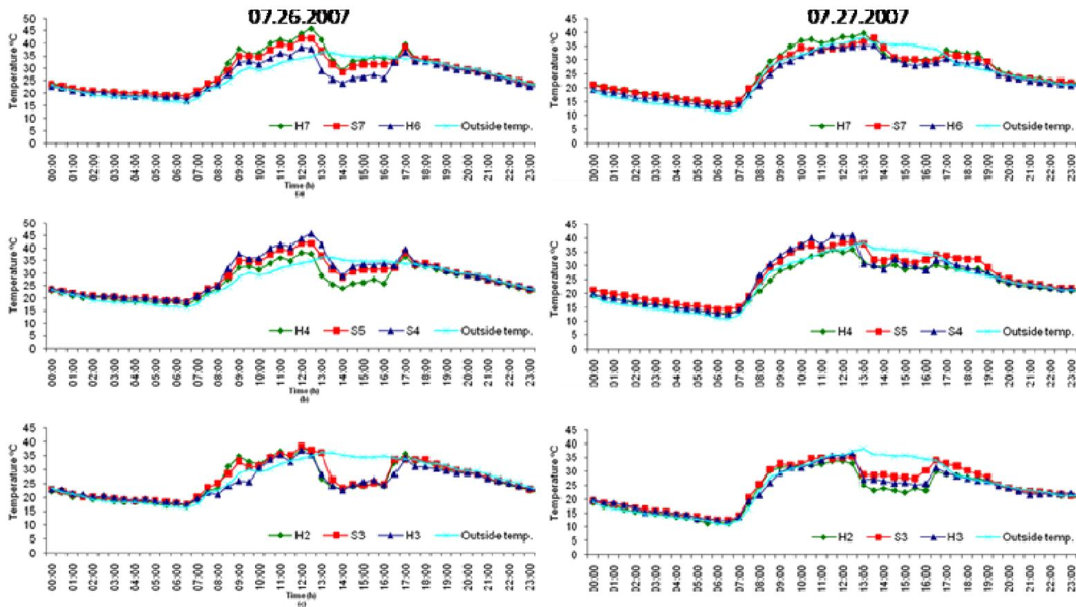
**Figure 3.** Hourly temperature changes of the sensors (a) in front of the fan, (b) in the center line, (c) in front of the pad; on July 26, 2007, when the outer relative humidity is the lowest and a day later (on July 27, 2007).
