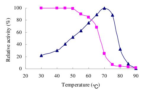
**Figure 7.** Optimal temperature (closed triangles) and thermostability (closed squares) of the xylanase from *S. chartreusis* L1105. The optimal temperature was determined at different temperatures and pH 7.2, MOPS buffer. To measure the thermostability, the xylanase in 50 mM MOPS buffer, pH 7.2, was incubated for 30 min at different temperatures.
