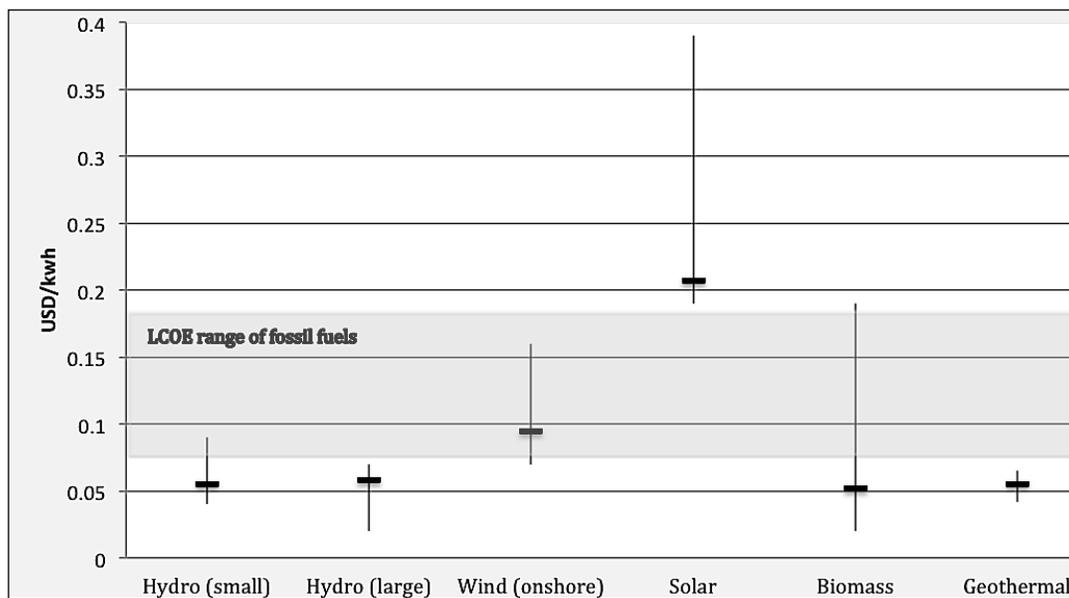
**Figure 3.** LCOE Ranges of Renewable Energy Technologies in Africa as compared to Fossil Fuels (for selected grid-connected projects). Source: IRENA 2013; IRENA 2012. Note: The horizontal black bars are the capacity weighted average value. Values for LCOE range of fossil fuels summarize ranges from South and East Africa as in IRENA 2013.
