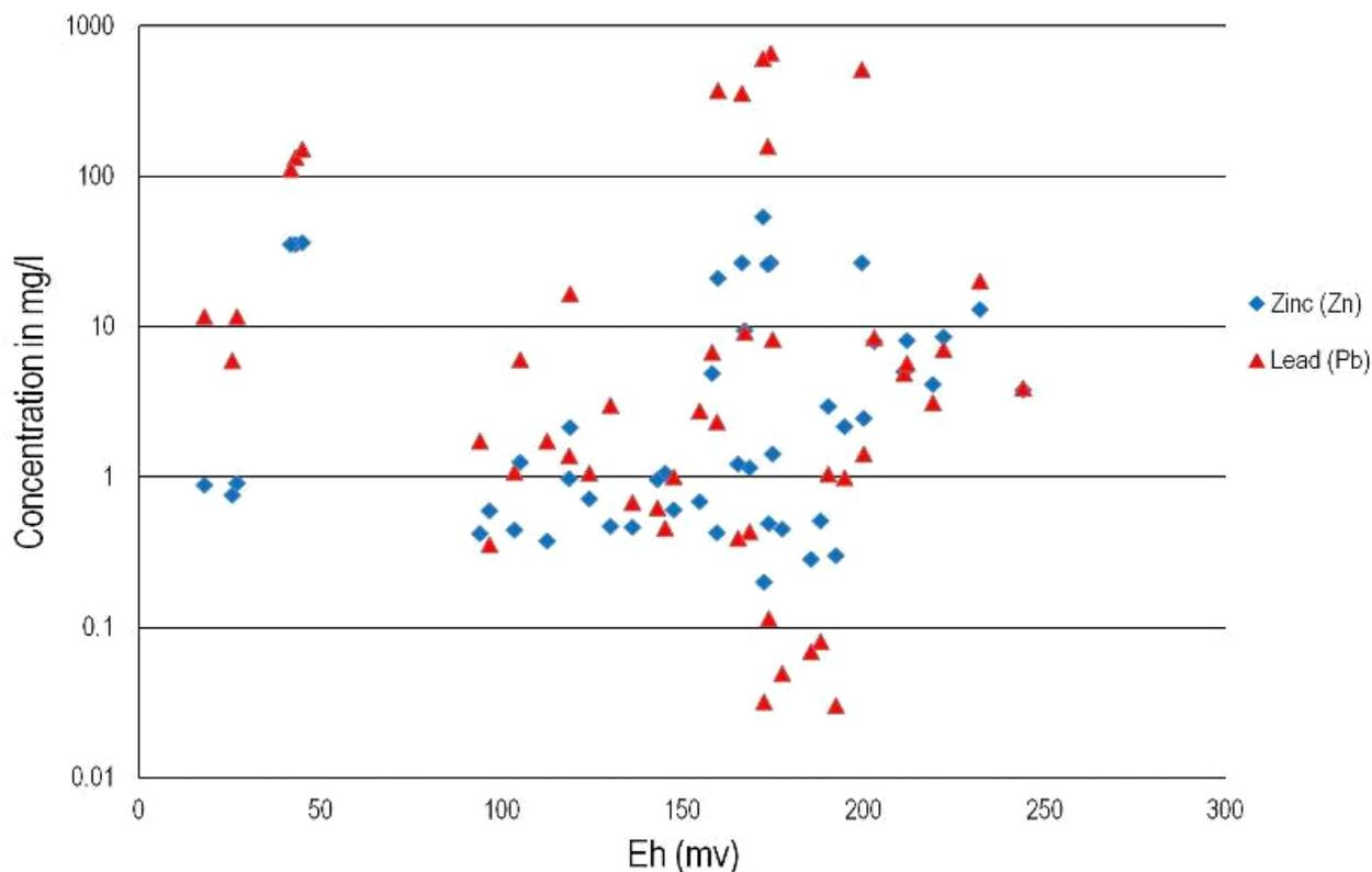
**Figure 5.** Leachability distribution of metals (Zn and Pb) as a function of oxidation reduction potential ( $E_h$ ) values regardless of leaching test methods (all tests were done in triplicate).
