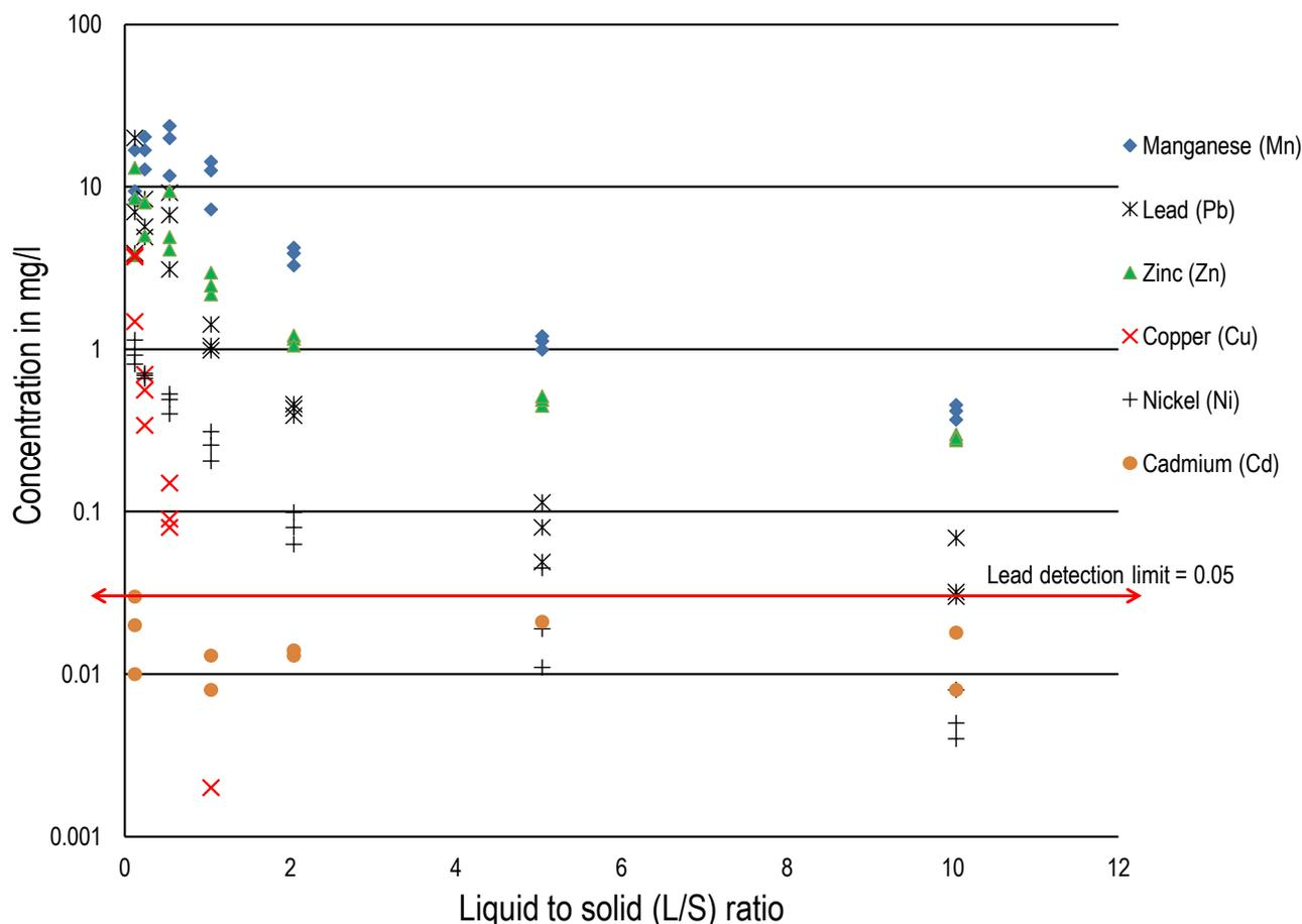
**Figure 1.** The solubility trend of Mn, Zn, Pb, Cu, Ni and Cd under the standard column leaching test conditions (tests were done in triplicate).
