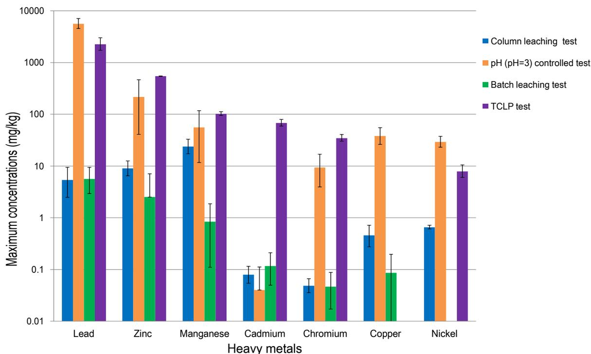
**Figure 4.** Maximum leachability (in mg/kg) of metals versus leaching test methods (all tests were in triplicate).
