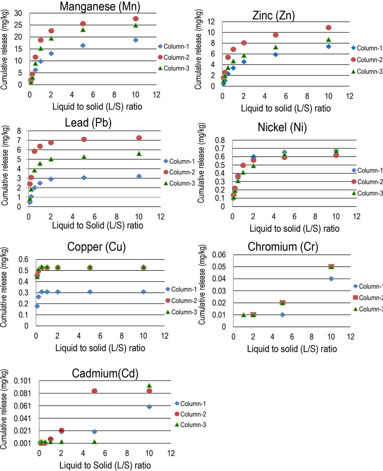
Figure 2. Cumulative release values of Mn, Zn, Pb, Ni, Cu, Cd and Cr from the three columns under the standard column leaching test conditions.
