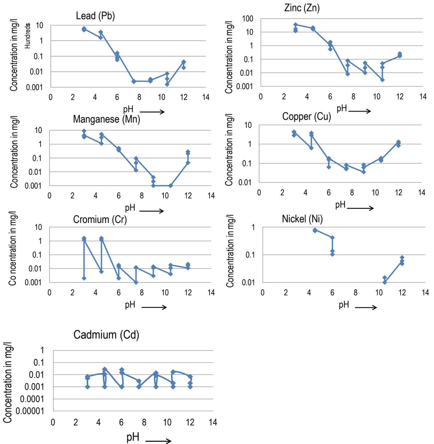
**Figure 3.** Leaching behavior of Pb, Zn, Mn, Cu, Ni, Cd and Cr as a function of pH (tests were done in triplicate).
