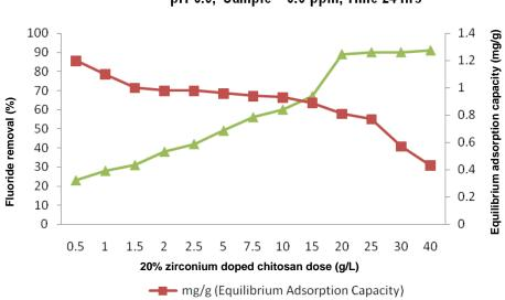
Effect of 20% Zirconium doped chitosan Dose on Defluridation , pH-6.9, Sample= 5.6 ppm, Time 24 hrs
