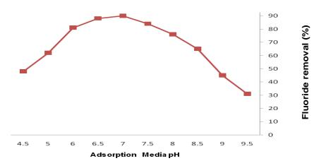
Figure 5. Effect of pH on fluoride adsorption using 20% Zr (IV) doped chitosan.
