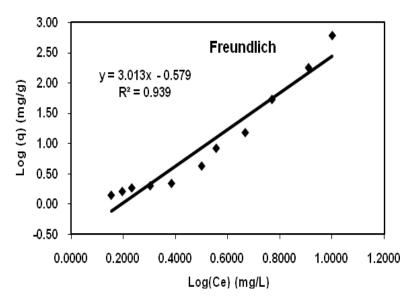
Figure 9. Freundlich adsorption isotherm for 20% Zr-chitosan composite.
