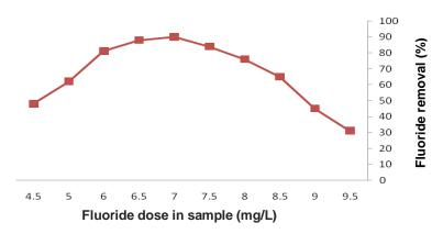
Figure 8. Effect of Initial Fluoride Concentration on fluoride removal, pH-6.9, time 24 h.
