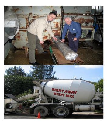
**Figure 3.** Top: Mr. Gusev demonstrates the way his mixing machine fills polyethyene tubes with the pasteurized, spawned substrate. Bottom: A concrete mixer that might be used for a pasteurization mixer. These are often available for used.
