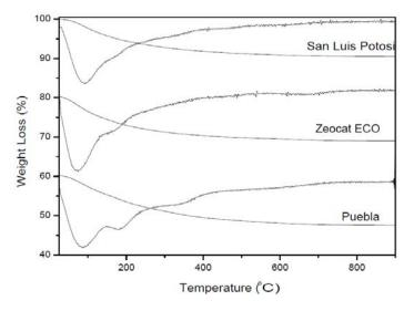
Figure 3. Thermogravimetric analyses of Mexican natural zeolites.
