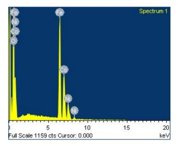
Figure 6. EDX spectrum of Ni<sub>0.25</sub>Co<sub>0.75</sub>Fe<sub>2</sub>O<sub>4</sub> nanoparticles.
