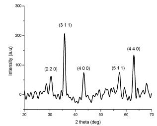
Figure 2. XRD pattern of Ni<sub>0.25</sub>Co<sub>0.75</sub>Fe<sub>2</sub>O<sub>4</sub> nanoparticles.
