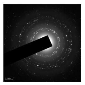
Figure 4. SAED pattern of Ni<sub>0.25</sub>Co<sub>0.75</sub>Fe<sub>2</sub>O<sub>4</sub> nanoparticles.
