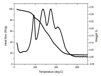
Figure 1. TG-DSC curve of Ni<sub>0.25</sub>Co<sub>0.75</sub>Fe<sub>2</sub>(cin)<sub>3</sub>(N<sub>2</sub>H<sub>4</sub>)<sub>5</sub>.
