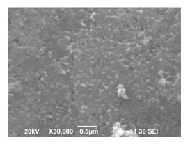
Figure 5. SEM image of Ni<sub>0.25</sub>Co<sub>0.75</sub>Fe<sub>2</sub>O<sub>4</sub> nanoparticles.
