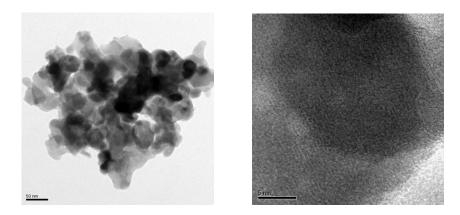
Figure 3. HRTEM image of  $Ni_{0.25}Co_{0.75}Fe_2O_4$  nanoparticles.
