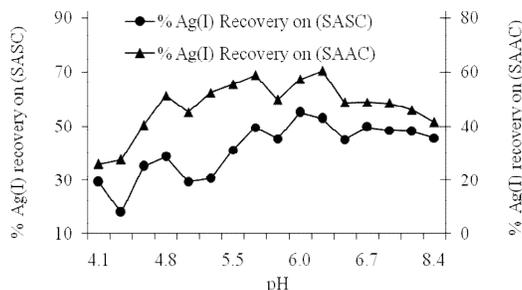
Figure 2. pH versus % cathodic Ag(0) recovery; cell voltage 1.5 V; all other parameters are same as for Figure 1.
