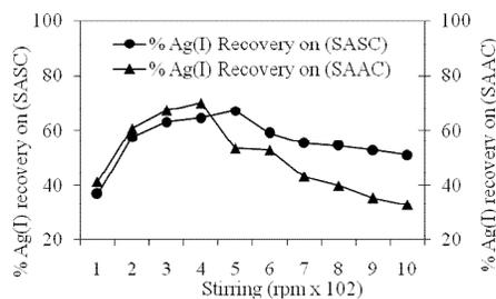
Figure 3. Stirring rate (rpm) versus % cathodic Ag(0) recovery; cell voltage 1.5 V; pH 6.1. All others parameters are same as for Figure 1.
