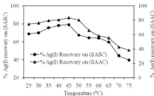
Figure 5. Temperature (°C) versus % cathodic Ag(0) recovery; cell voltage 1.5 V; pH 6.1; stirring rate, 400 rpm. All others parameters are same as for Figure 1.
