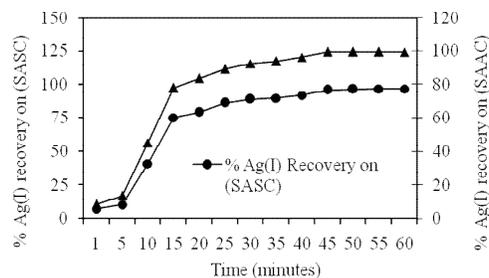
Figure 6. Electrolysis time (min) versus % cathodic Ag(0) recovery; temperature,  $45 \pm 1$  °C; cell voltage 1.5 V; pH 6.1; stirring rate, 400 rpm. All others parameters are same as for Figure 1.
