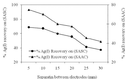
Figure 4. Separation between electrodes (mm) versus % cathodic Ag(0) recovery; cell voltage 1.5 V; pH 6.1; stirring rate, 400 rpm. All others parameters are same as for Figure 1.
