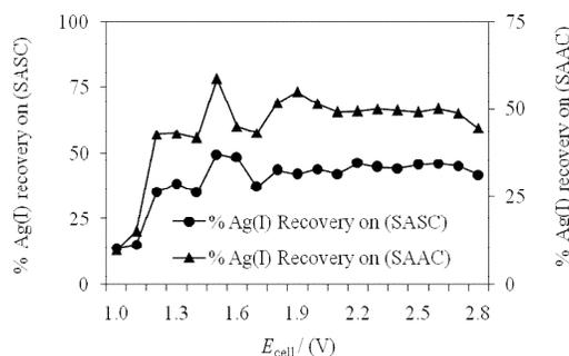
Figure 1. Cell voltage (V) versus % cathodic Ag(0) recovery; a set of electrodes couples (SASC) and (SAAC); Ag(I) concentration, 100  $\mu\text{g/mL}$ ; pH,  $5.7 \pm 0.1$ ; depth area of electrode,  $1.9 \times 3.7 \text{ cm}^2$ ; separation between electrodes 1cm; deposition time, 20 min; temperature,  $25 \pm 1 \text{ }^\circ\text{C}$ ; stirring rate, 200 rpm; 0.2 M acetate buffer with 0.005 M  $\text{NH}_3$  as supporting electrolytes and pH adjuster.
