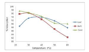
Figure 6. Effect of temperature on Ni(II) removal (30 mg/L, 1.5 g leaf, 250 rpm agitation speed, 90 min time and pH of 5 for leaf, at 20 mg/L, 2 g bark, 250 rpm agitation speed, 120 min time and pH of 6 for bark and also at 50 mg/L, 2.5 g seed, 300 rpm agitation speed, 90 min time and pH of 6 for seed).
