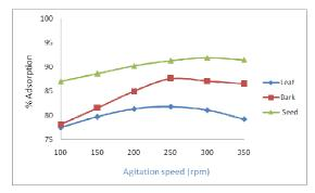
Figure 3. Effect of agitation speed for Ni(II) removal (room temperature, 30 mg/L, pH of 2.5, 1.5 g leaf and 60 min time for leaf, at room temperature, 20 mg/L, pH of 2.5, 2 g bark and 60 min time for bark and also at room temperature, 50 mg/L, pH of 2.5, 2.5 g seed and 60 min. time for seed).
