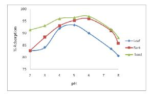
Figure 5. Effect of pH on Ni(II) removal (30 mg/L, 1.5 g leaf, 250 rpm agitation speed, 90 min. time and room temperature for leaf, at 20 mg/L, 2 g bark, 250 rpm agitation speed, 120 min. time and room temperature for bark and also at 50 mg/L, 2.5 g seed, 300 rpm agitation speed, 90 min. time and room temperature for seed adsorbent).
