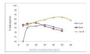
Figure 1.Effect of initial concentration on Ni(II) removal (1 g adsorbent, 250 rpm agitation speed, pH of 2.5, 60 min contact time and room temperature for each adsorbent).
