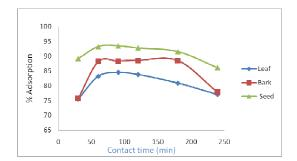
Figure 4. Effect of contact time for Ni(II) removal (30 mg/L, 1.5 g leaf, pH of 2.5, 250 rpm agitation speed and room temperature for leaf, at 20 mg/L, 2 g bark, pH of 2.5, 250 rpm agitation speed and room temperature for bark and also at 50 mg/L, 2.5 g seed, pH of 2.5, 300 rpm agitation speed and room temperature for seed).
