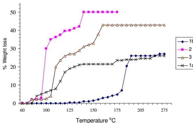
Figure 1. Thermogravimetric analyses of complexes **1a**, **1b**, **2** and **3**.
