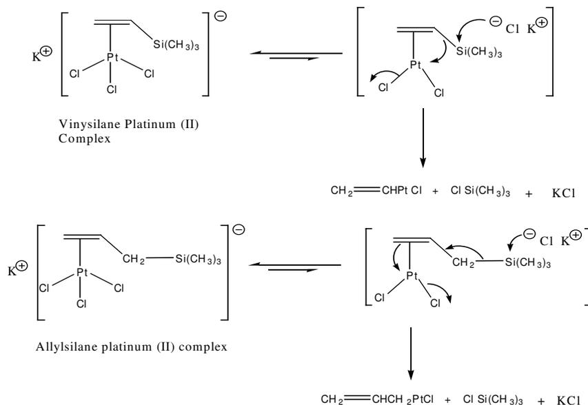
Scheme 1. Proposed mechanisms for the thermal decomposition of vinyl- and allylsilane platinum(II) complexes.
