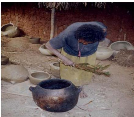
**Picture 3** Pot under post firing treatment
