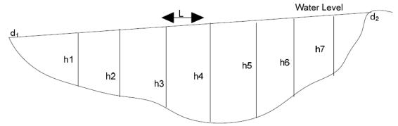
Figure 3.6: Cross Section of a Drainage Channel
