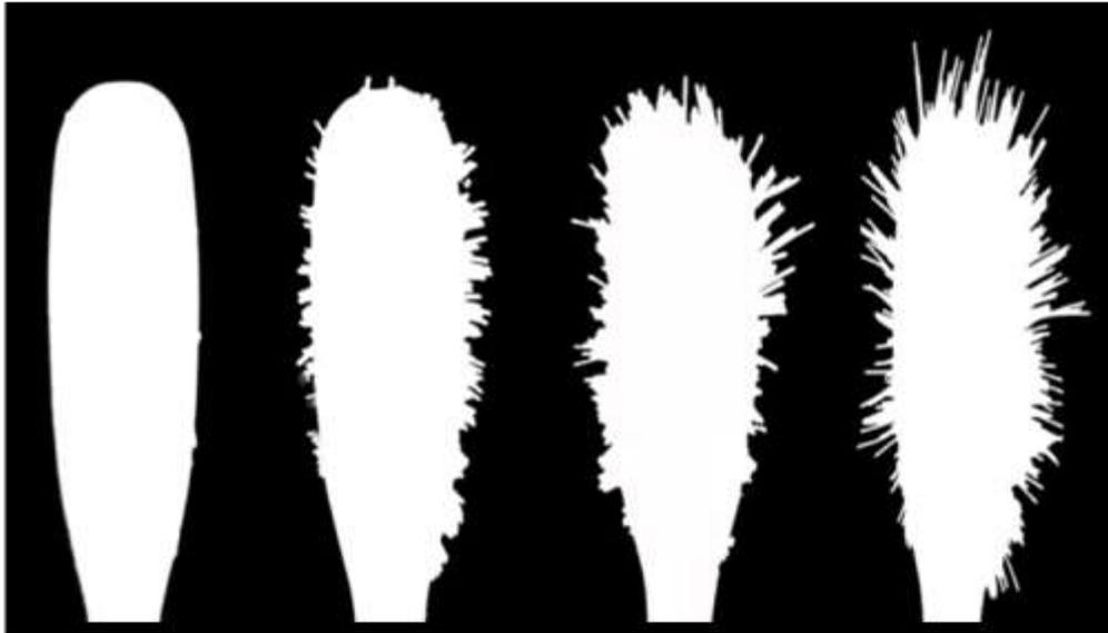
Figure 2: Various entanglement styles and splaying observed in tooth brushes
