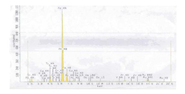
**Figure 7**: Energy dispersive X-ray spectrum of Okaba coal seam 4 samples at 20m depth from open pit mine site.
