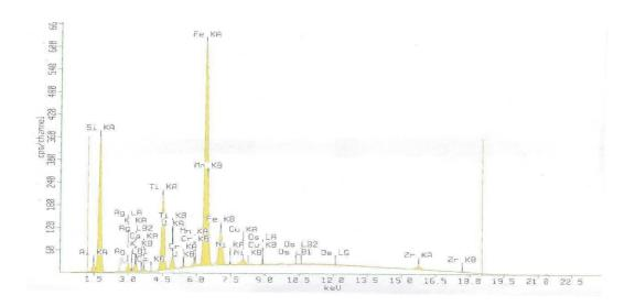
**Figure 4**: Energy dispersive X-ray spectrum of Okaba coal seam 1 samples: 5m depth from Open pit mine.
