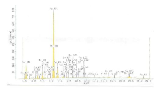
**Figure 10**: Energy dispersive X-ray spectrum of shale 2 samples 10m above coal deposits from open pit mine site.
