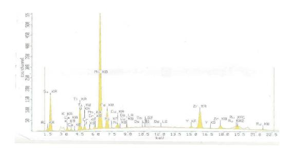
**Figure 9**: Energy dispersive X-ray spectrum of shale 1 sample 5 m above coal deposits from Open pit mine at Okaba.
