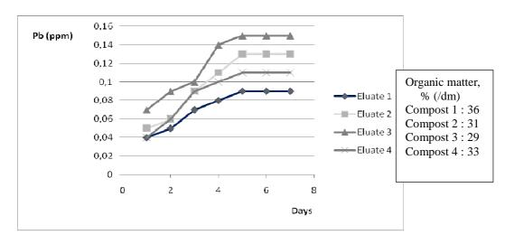
Figure 2: Extraction of Pb with EDTA (0,05M) pH=7.
