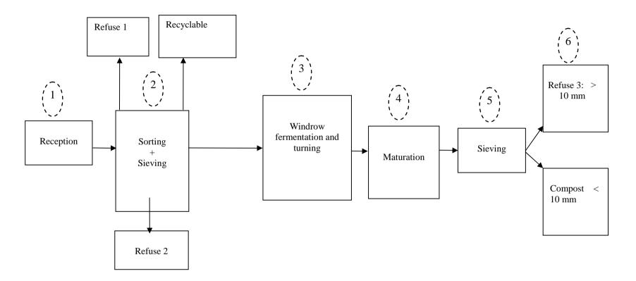
Figure 1: Plan of the line in industrial scale composting. Refuse 1: > 10 mm, no recyclable; Refuse 2: < 10 mm, 90 % of sand.
