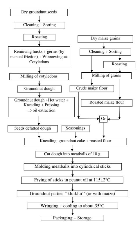
Figure 1: Flow chart of the groundnut patties manufacturing process.
