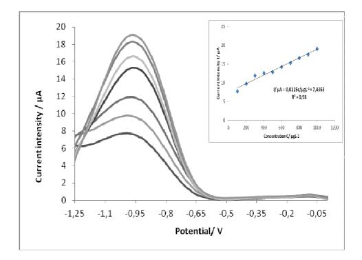
**Figure 4:** Analytical curves for glyphosate herbicide in Glyphonet SL 360 formulation determination in the concentration range of 100 to 1000  $\mu$ g L<sup>-1</sup> in pH 5.2 phosphate buffer solution using carbon fiber microelectrode. Reference electrode: Ag/AgCl 0.1 M KCl. Frequency: 60 Hz. Scan increment: 10 mV. Pulse height: 60 mV.
