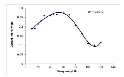
**Figure 3:** Evolution of the current intensity of the reduction of glyphosate with the frequency in pH. 5.2 phosphate buffer solution using carbon fiber microelectrode working electrode and an Ag/AgCl/KCl 0.1 M as reference electrode.
