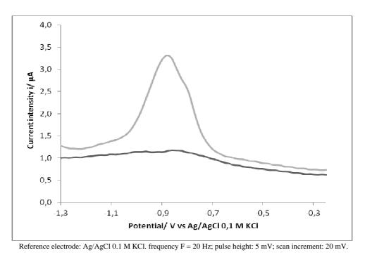
**Figure 1:** Square wave voltammograms of phosphate buffer solution pH 5 (black) and 40  $\mu$ g L<sup>-1</sup> of glyphosate (grey) using CFME ( $\Box \Phi = 12 \mu$ m).
