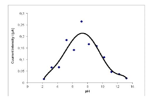
**Figure 2:** pH effect on the current intensity of the glyphosate reduction using CFME ( $\Phi = 12 \mu m$ ). Reference electrode: Ag/AgCl 0.1 M KCl, frequency 10 Hz, scan increment: 5 mV and pulse height: 20 mV.
