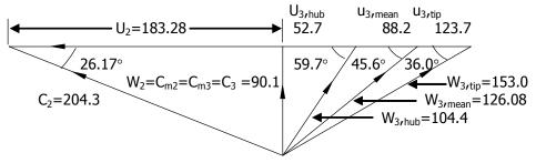
Figure 6: Velocity diagrams for expansion turbine (All velocities are in units of m/s)
