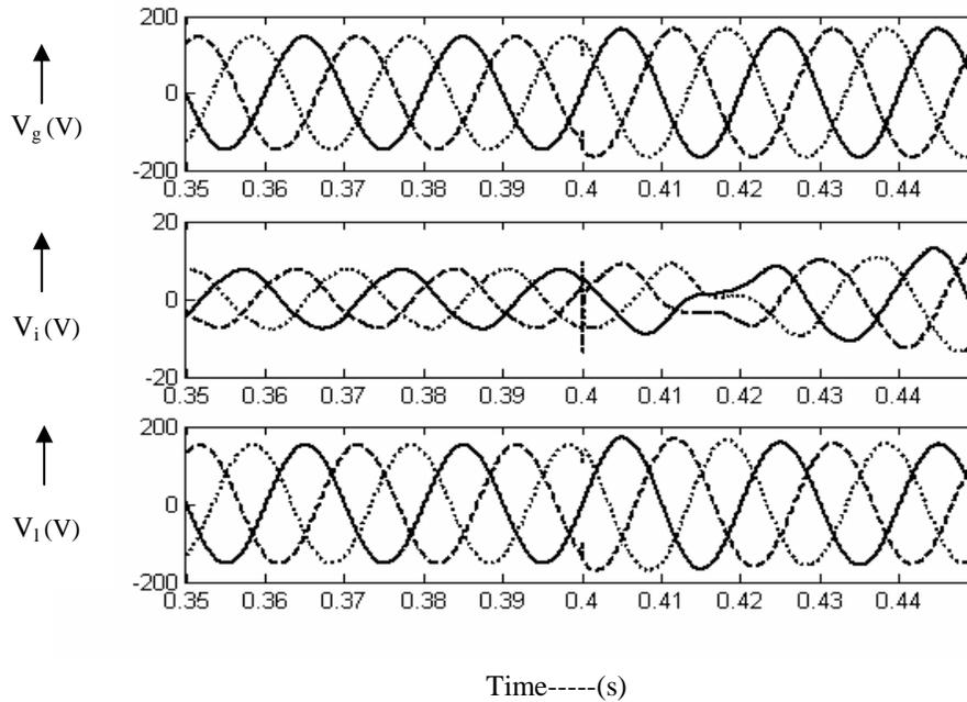
Figure 10: Waveforms of source voltage, injected voltage and load voltage under 3-phase case
