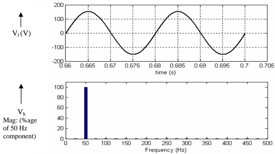
Figure 9 : Harmonic analysis of load voltage
