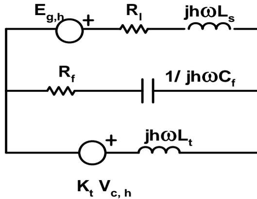
Figure 3: Single-phase  $h_{th}$  harmonic equivalent circuit
