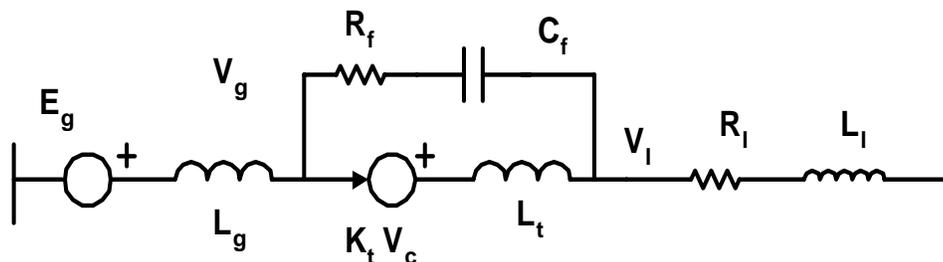
Figure 2 : Harmonic filter connected on line side (i.e., across the secondary of injected transformer)
