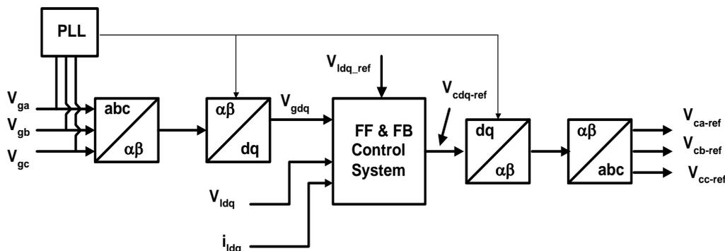
Figure 5: Final control scheme of DVR under feedback and feedforward control scheme
