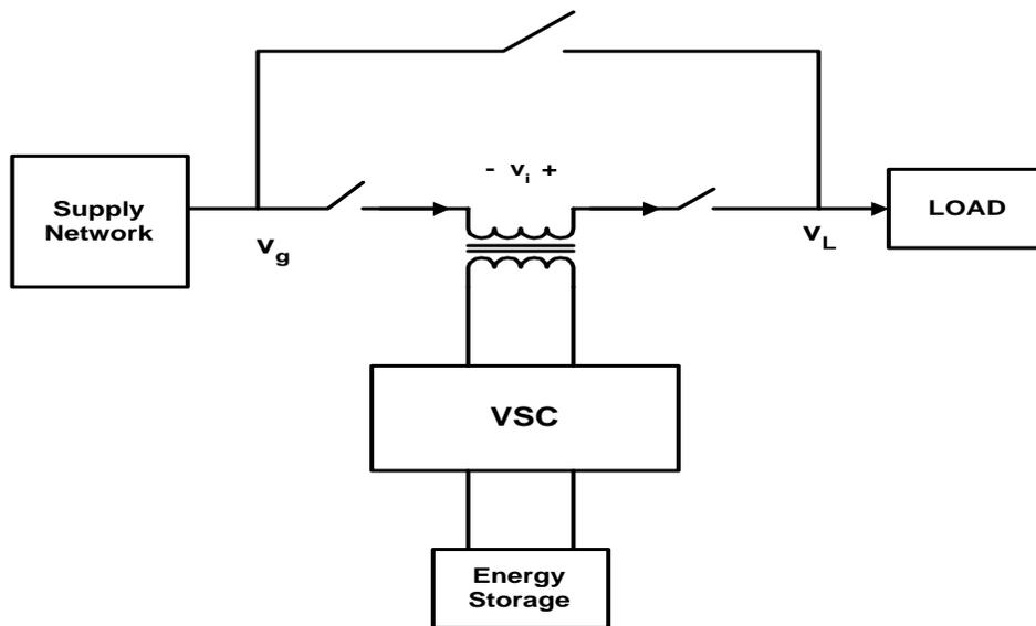
Figure 1. Basic Structure of DVR
