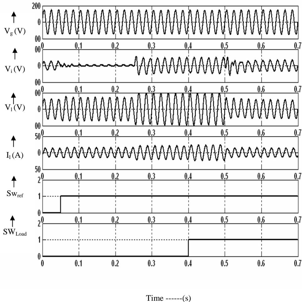
Figure 7: Waveforms of source voltage, injection voltage, load voltage, load current, instant of change in load reference command and instant of load switch for change in load
