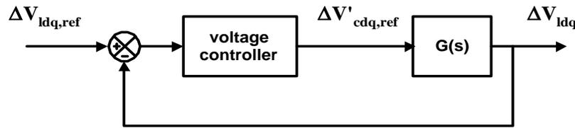
Figure 4: Feedback control loop of DVR
