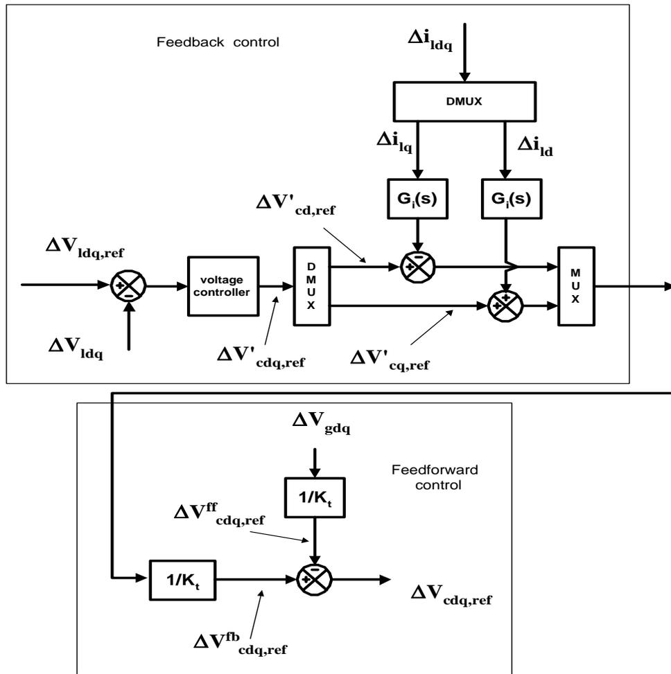
Figure 6: Feedback and feedforward control scheme
