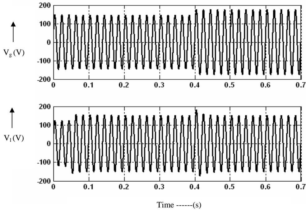
Figure 8 :Wave forms of source voltage and load voltage under variation in input voltage and reference command
