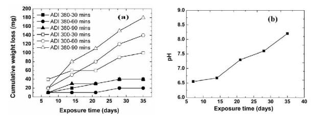
Figure 3(a) Cumulative weight losses versus exposure time for different samples, (b) Variation in pH of the iron ore slurry with time
