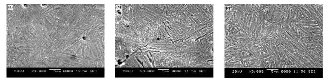
Figure 1b. Microstructure of ADI, austempered at 300 C. (a) 30 mins (b) 60 mins (c) 90 mins.
