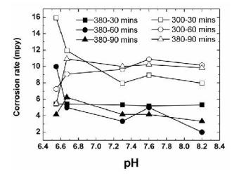
Figure 4 Variations in corrosion rate of (a) high temperature ADIs and (b) low temperature ADIs as a function of pH of the iron ore slurry
