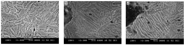
**Figure 1a.** Microstructure of ADI, austempered at 380 C. (a) 30 mins (b) 60 mins (c) 90 mins.
