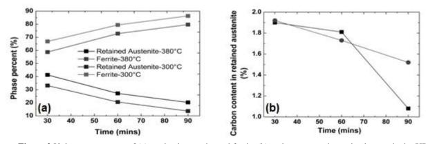
Figure 2 Volume percentage of (a) retained austenite and ferrite (b) carbon content in retained austenite by XRD analysis
