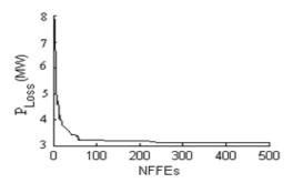
Figure 3. Convergence profile of  $P_{Loss}$  for  $P_{Loss}$  minimization objective of modified IEEE 30-bus system
