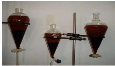
Fig. 1. Biodiesel separation flask
