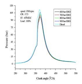
Fig. 15: Effect of IP on Peak pressure at 100% load.
