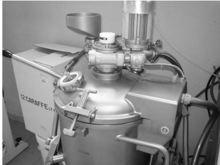
Figure- 3 Refrigerated vacuum milling chamber
