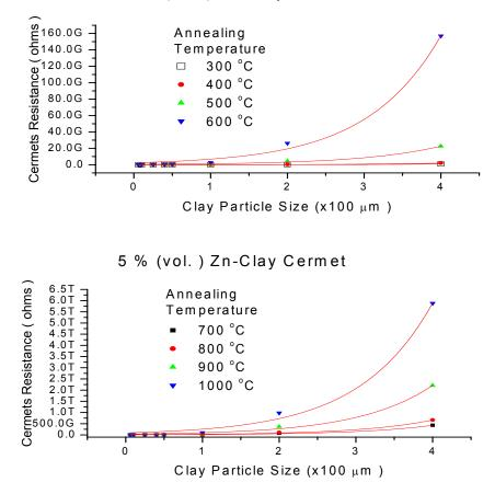
Fig. 1 Variation of Cermets Resistance with Clay Particle Size for 5 % (vol.) Zn- Clay ratio.
