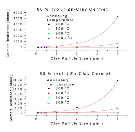
Fig. 2 Variation of Cermets Resistance with Clay Particle Size for 60% (vol.) Zn- Clay ratio.
