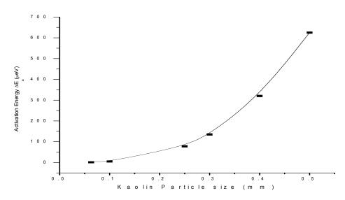
Fig. 3 Variation of Activation Energy with kaolin particle size for 60% (vol.) Zn composite resistors.
