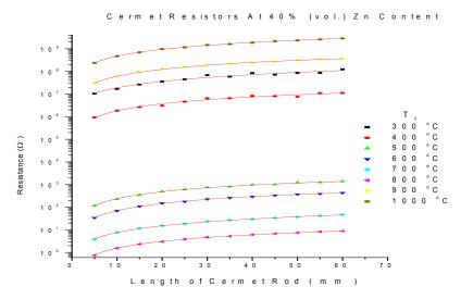
Fig. 6 Variation of Cermet resistance (emphasizing the effect of annealing Temperature) with resistor length for Zn concentration = 40%(vol.)Zn
