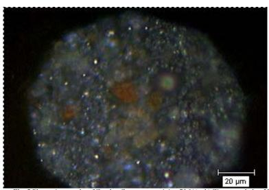
Fig. 5 Photomicrographs of Zn-clay Cermets containing 70 %(vol.) Zinc annealed at 500
