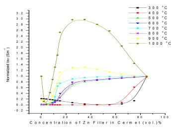
Fig. 4 Variation of Normalized Inσ with Filler concentration showing the variation of percolation threshold with annealing temperature
