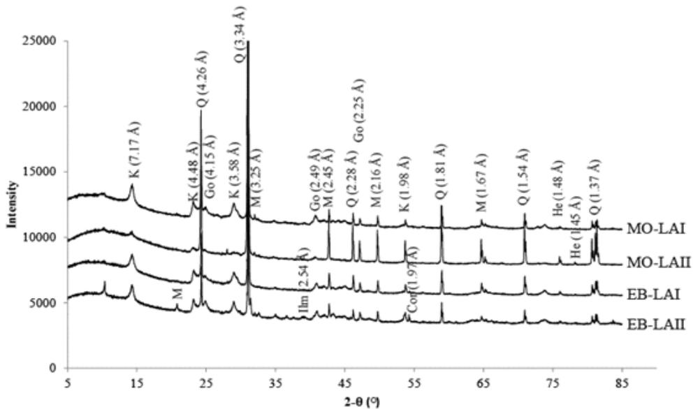
Fig. 3. X-ray diffraction pattern of the lateritic clays of Monatele and Ebebda
