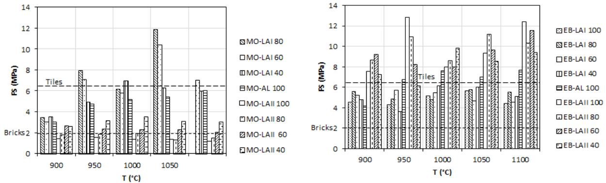
Fig. 7. Flexural strength variation with firing temperature of Monatele and Ebebda tested bricks
