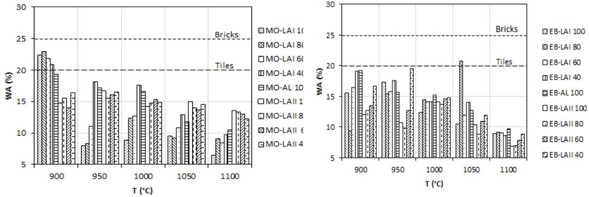
Fig. 6. Water absorption variation with firing temperature of Monatele and Ebebda tested bricks
