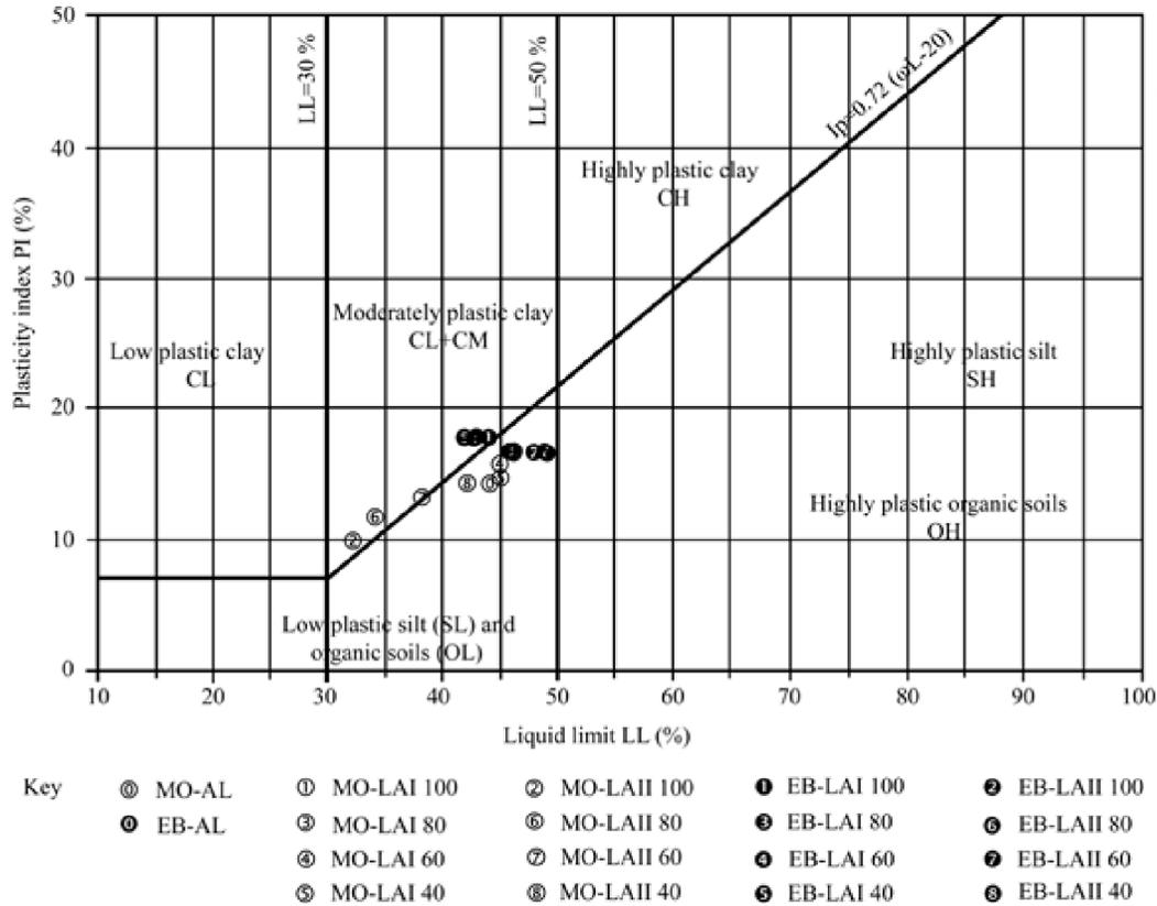
Fig. 4. Position of Monatele and Ebebda clays in the Casagrande plasticity chart
