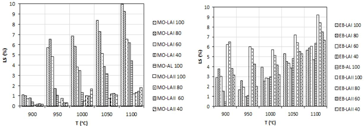
Fig. 5. Linear shrinkage variation with firing temperature of Monatele and Ebebdba tested bricks
