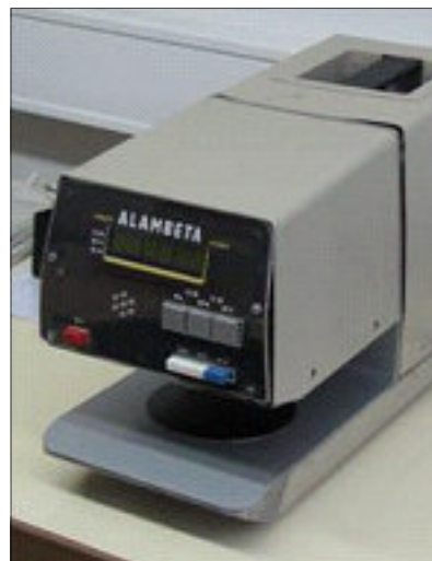
FIGURE 2: PHOTOGRAPH OF THE ALAMBETA TEST INSTRUMENT
