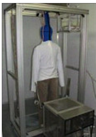
FIGURE 1: PHOTOGRAPH OF THE WALTER™ – SWEATING THERMAL MANIKIN
