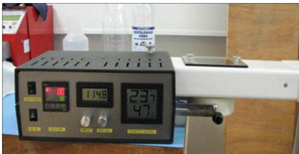
FIGURE 3: PHOTOGRAPH OF THE PERMETEST TEST INSTRUMENT
