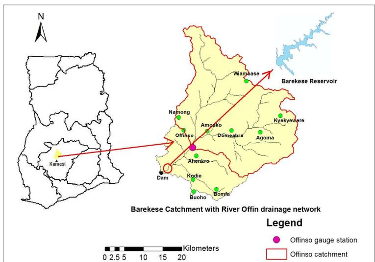
**Fig. 1: Location of Barekese Reservoir, dam and catchment area with River Offin drainage network**
