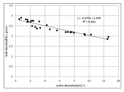
Figure 6. Water absorption versus bulk density.
