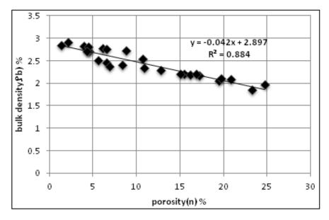
Figure 5. Graph showing Porosity versus bulk density.
