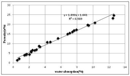
Figure 4. Linear relationship between porosity and water absorption of all the ignimbrite and rhyolitic tuff volcanic rocks.
