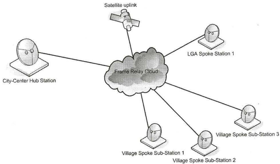
Figure 1.6 *Frame relay network topology cloud*
