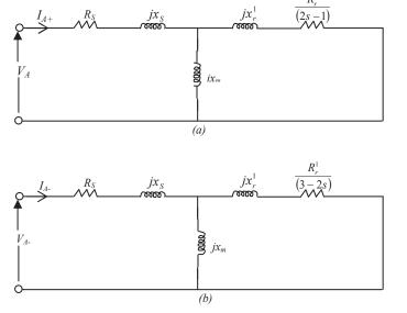
Figure 5: Per phase-sequence networks of the 3-phase TF machine (a) Positive (b) Negative.
