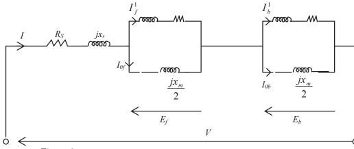
Figure 6: Equivalent circuit of a single phase transfer field machine for any slip s.
