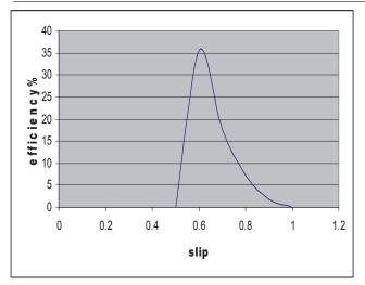
Figure 8: Efficiency/slip curve of SPTF machine.
