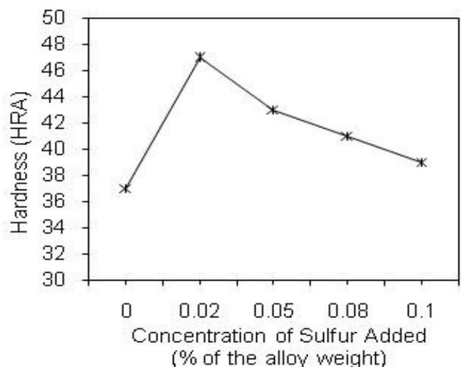
Figure 7: Variation of Hardness of Al-12wt%Si sand cast alloy with sulphur addition.
