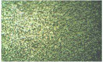
Micrograph A5: Micrograph of 0.509% carbon steel quenched in cotton seed oil, showing low proportion of martensitic structure (dark) in ferric (white) matrix x 200.
