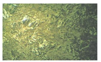
Micrograph A2: Microstructure of water quenched microstructure of 0.509% carbon steel showing martensite structure (dark) with retained austenite (white) x 200.
