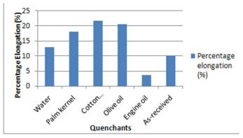
*Figure 3: Percentage Elongation values of the medium carbon steel sample in different quenchants.*
