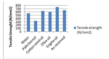
*Figure 2: Tensile Strength values of the medium carbon steel sample in different quenchants.*
