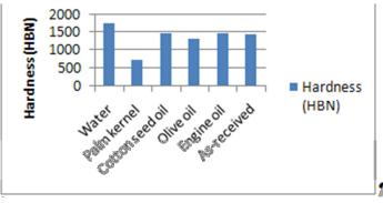
*Figure 5: Hardness values of the medium carbon steel sample in different quenchants.*
