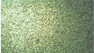
*Micrograph A4: Micrograph of 0.509% carbon steel quenched in palm kernel oil, showing low proportion ofmartensite structure (dark) in ferric (white) matrix x 200.*
