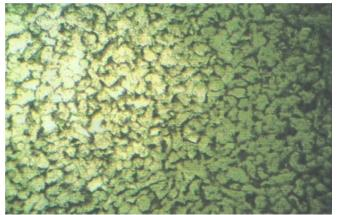
*Micrograph A1: Microstructure of as-received structure of 0.509% carbon steel showing pearlite (dark) in ferric (white) matrix x 200*
