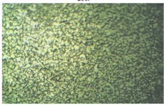
*Micrograph A6: Micrograph of 0.509% steel quenched in olive oil, showing low proportion of martensitic structure (white) with retained austenite (dark).*
