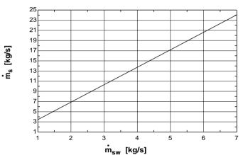
*Figure 4: Changes in the quantity of steam generated in relation to amount of solid waste combusted.*
