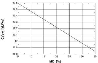
*Figure 3: Variation of calorific value of the solid waste with different values of moisture content.*
