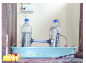
Figure 1: Microbial Fuel Cell for the treatment of waste water
