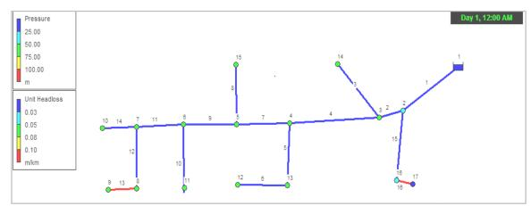
Figure 2: Water distribution network, EPANET result
