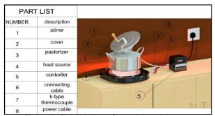
Figure 1: Pictorial view of experimental set-up
