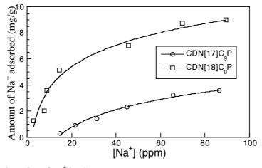
**Figure 4:** Adsorption of  $Na^+$  by SPP.
