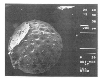
Figure 2: A magnified polymer particle from CNSL
