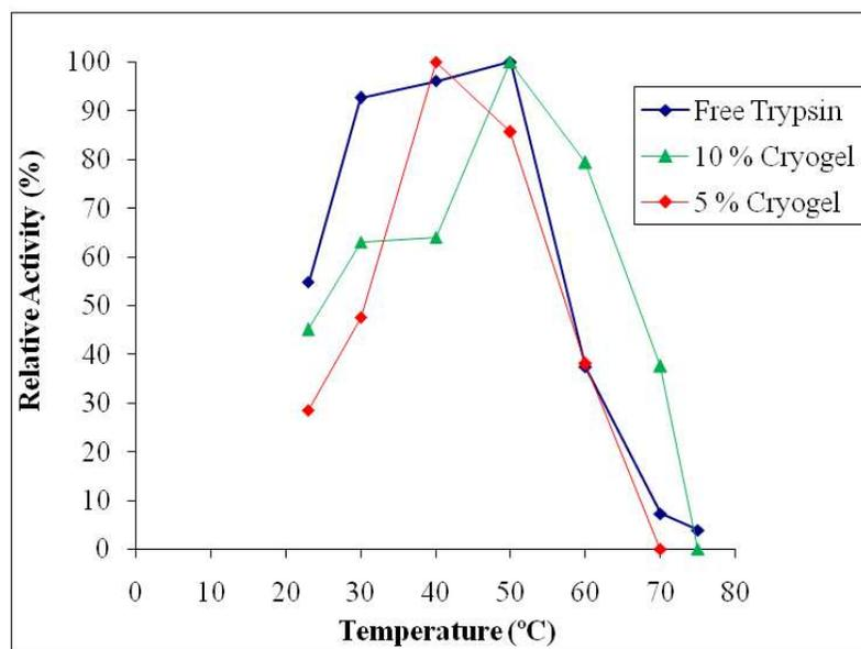
**Figure 5:** Effect of temperature on activity of free trypsin and epoxy-MPAAG immobilized trypsin
