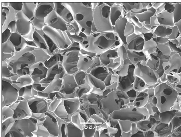
**Figure 1:** SEM image for 10 % poly(epoxyacrylamide) cryogel.
