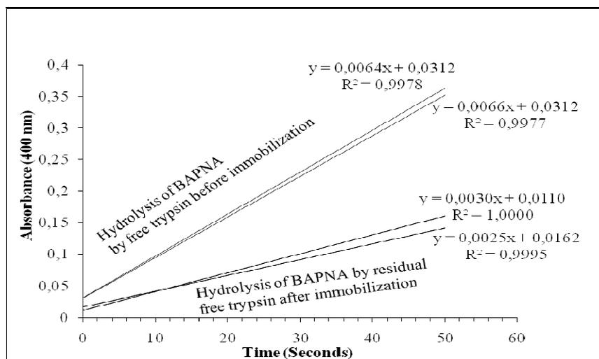
**Figure 2:** Absorbance v/s Time Graphs: Estimation of Initial Rates of Hydrolysis of BAPNA for the Determination of the Activity Based Immobilization Yield for the 10 % Epoxy-MPAAGs Cryogel-Trypsin Conjugates.
