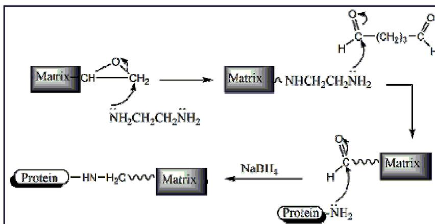
**Scheme 2:** Reaction Scheme for Covalent Attachment of Trypsin onto the Epoxy-MPAAGs Cryogels using Ethylenediamine and Glutaraldehyde; Followed by Reduction of the Schiff Base by Sodium Borohydride (Petro *et al.* 1996).
