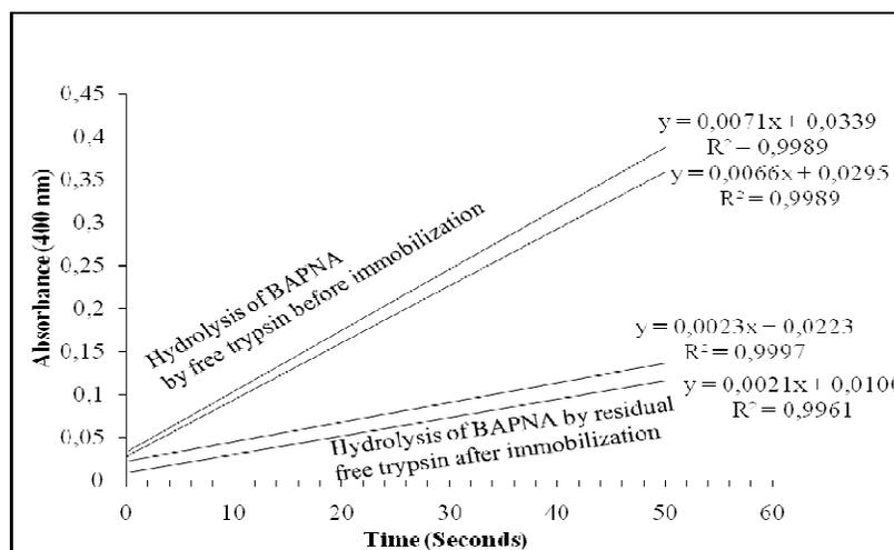
**Figure 3:** Absorbance v/s Time Graphs: Estimation of Initial Rates of Hydrolysis of BAPNA for the Determination of the Activity Based Immobilization Yield for the 15 % Epoxy-MPAAGs Cryogel-Trypsin Conjugates.
