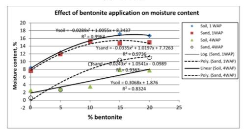
Figure 1. Effect of bentonite application on the moisture content of different soil types.
