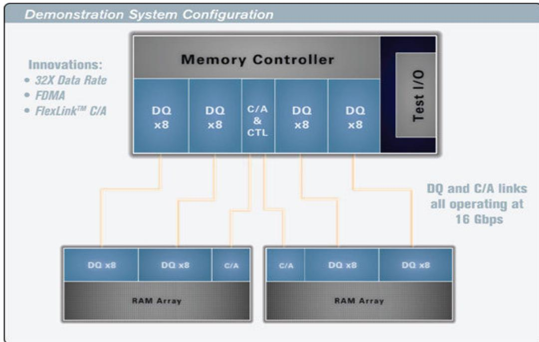
**Fig. 2: The Rambus Terabyte Bandwidth Initiative**
