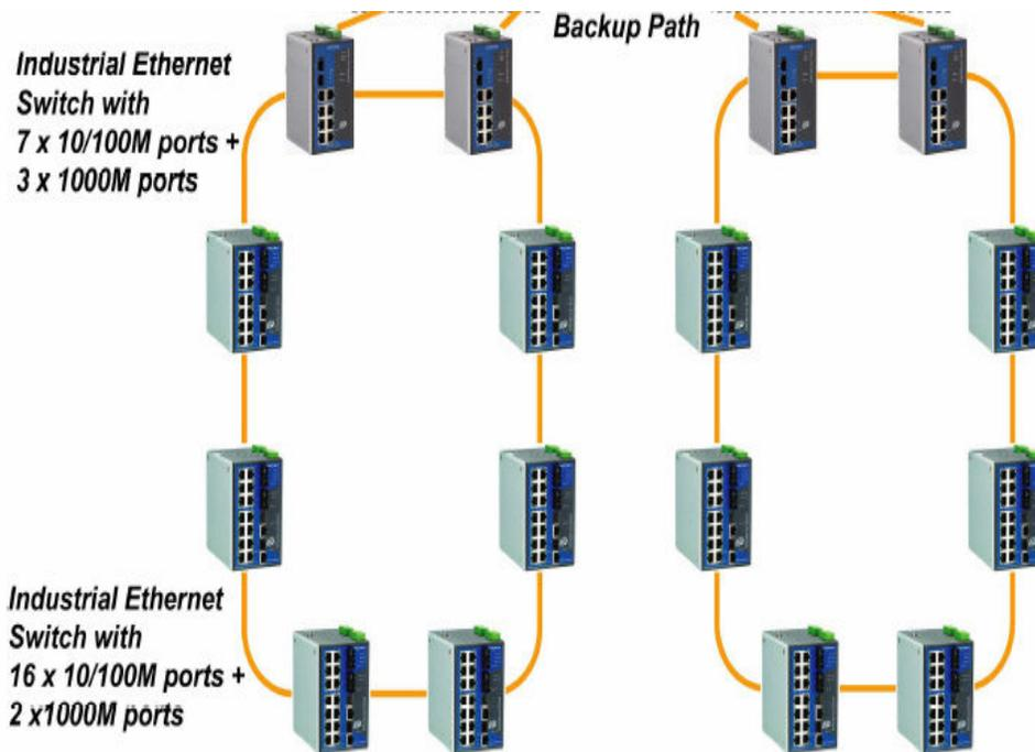
**Fig. 1b Network Diagram of the proposed Redundant Gigabit Backbone for the case study**
