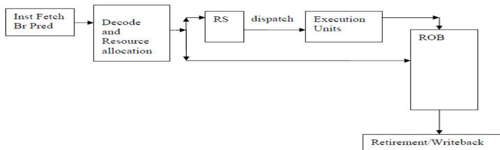
**Figure 4 Block Diagram of Out of Order Execution**
