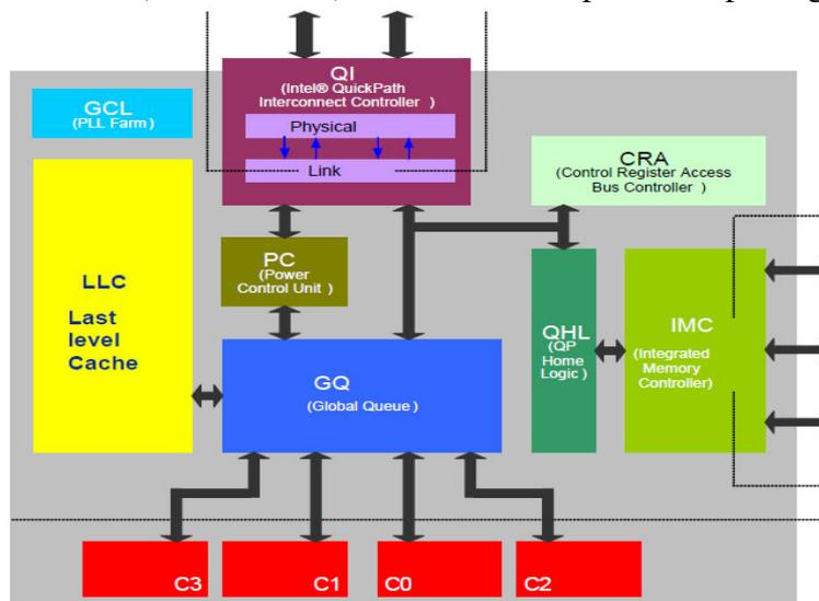
Figure 5 block diagram of the Intel® Xeon™ 5500 processor
