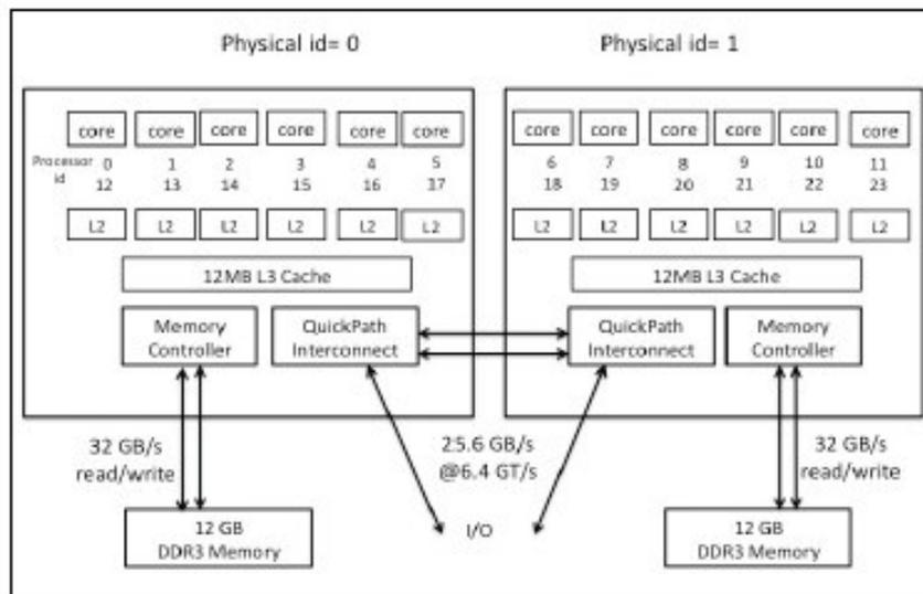
**Figure 2. Configuration of an Intel Westmere-EP node.**
