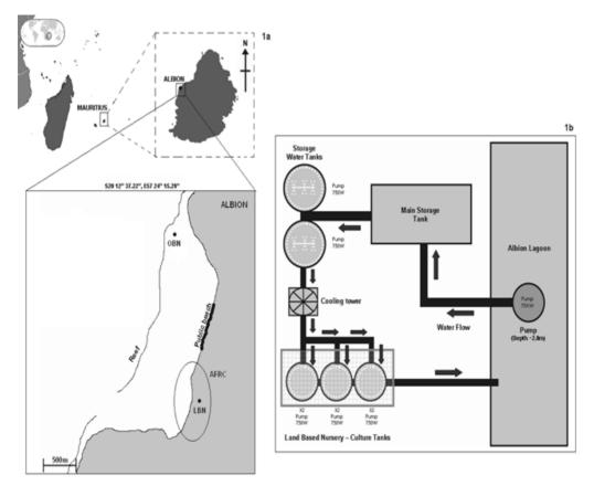
Figure 1. a) Site location of the Land-Based (LBN) and Ocean-Based Nurseries (OBN) in Mauritius and b) schematic representation of the LBN set up at Albion.
